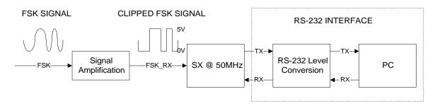
Demonstrating FSK detection requires this type of circuitry, in addition to some means of creating the FSK signal. Integrating this type of solution into an operational modern would require one additional block: the isolation circuitry, which isolates the outside phone line from the modern's internal analog circuitry. There are standard isolation circuits for every country, so check with the local standards committee.
